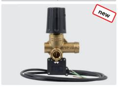
⊕ = Inlet 3/8" F. ⊖ = Outlet 3/8" F. BP = Bypass 3/8" F. Check valve with conical-piston. By-pass valve with switch (IP6K7) and cable 1,200 mm. Max. 250 bar / 80 °C
