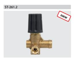
© = Inlet 3/8" F. © = Outlet 3/8" F. BP = Bypass 3/8" F. check valve with plastic valve cone. Max. 250 bar / 80 °C
