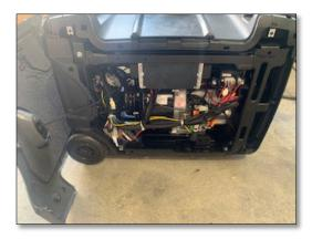
2. Remove the bolts for the front face, there are 4 on the front and 2 from the top and each side.
