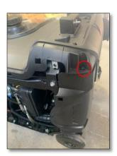
3. Fit the main box as pictured. It is a tight fit and the engine may need to be pushed on the rubber mounts to allow space for the bolt to be fitted into the slot.
